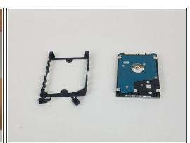
Peel off the rubber hard drive mount.
