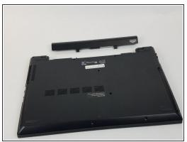
Pull the battery out, keeping it flat and parallel to the laptop so that it slides out easily.
