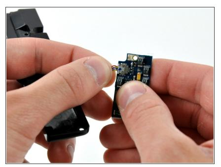
• Disconnect the audio-out cable by pulling the male end straight away from its socket on the audio board.
