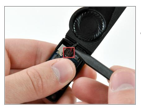
Use the tip of a spudger to pry the speaker connector up off the audio board.
