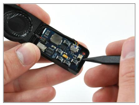
• Use the tip of a spudger to separate the audio board from the adhesive securing it to the logic board.
