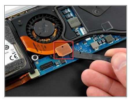
Use a spudger to pry the hard drive cable connector up off the logic board.
