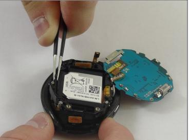
• Using <u>tweezers</u>, lift the battery casing.
