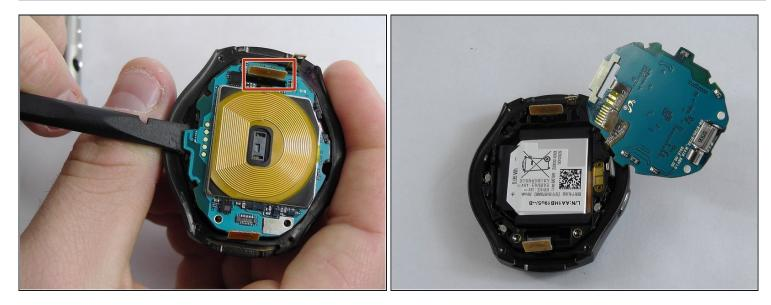
Using the flat end of a spudger, pry up the motherboard.
