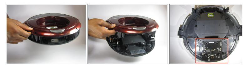
• To access the motherboard, lift the top portion of the vacuum off.
