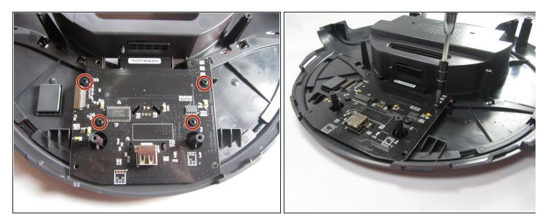
Use a Phillips #1 screwdriver to remove the four 10 mm screws holding the motherboard in place.
