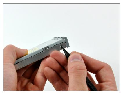
Use the tip of a spudger to depress and release the bezel retaining tab on the side of the optical drive.
