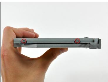
• Remove the two 4.5 mm shouldered T6 Torx screws from each side of the optical drive (four screws total).
