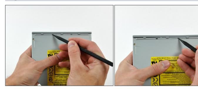
Use the tip of a spudger to push the two plastic bezel tabs away from their retaining slots on the top of the optical drive.
