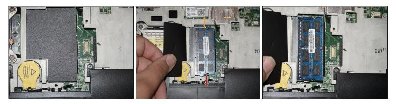
• To remove the RAM module, follow the removal procedure from the bottom lower module.
