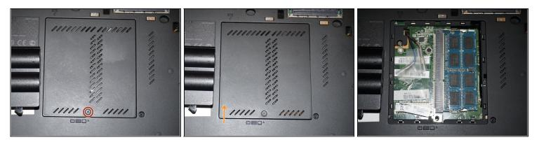
• To remove the bottom memory module, open the memory door. Use a *Phillps #0* screwdriver.
