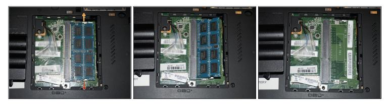
• With the bottom RAM door removed, release the bottom memory module. Release both locking tabs and the module can be removed.
