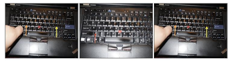
• To remove the keyboard, push up from the bottom first. Once the lower tabs are released, use a plastic pry tool to lift the keyboard up.
