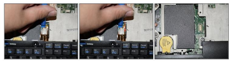
• Once the keyboard is removed, disconnect the cable from the motherboard. Use a plastic pry tool.
