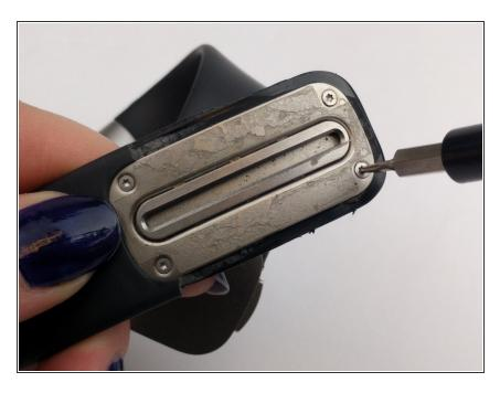
Use a T3 Torx screwdriver to unscrew the four 6 mm screws on the corners of the metal cover plate.
