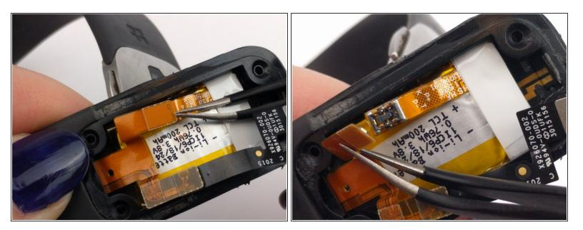
Detach the orange press-fit (or "pop") connector by using the tweezers.
