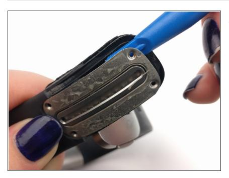
Use the plastic opening tool to pry off the metal cover plate.
