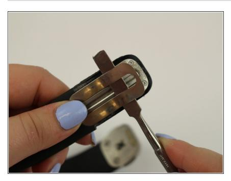
Peel back the metal cover on the end of the watchband.
