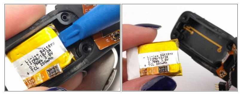
Pry out the battery using the plastic opening tool.
