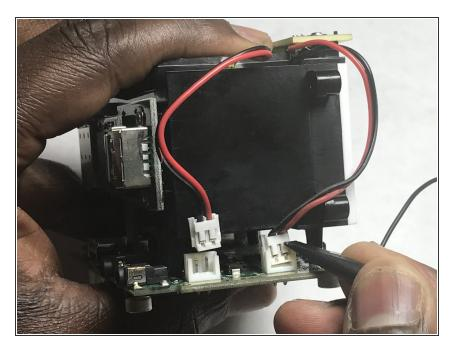
Remove the Chumby button connector using a plastic spudger.
