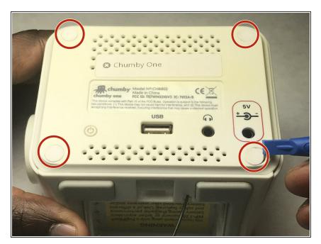
Remove 4 self-adhesive plastic dots covering the screw holes.
