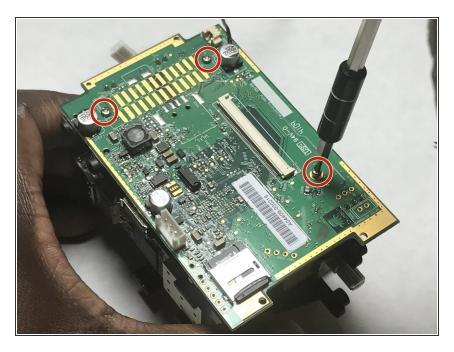
Remove three 6mm screws using a PH000 bit.
