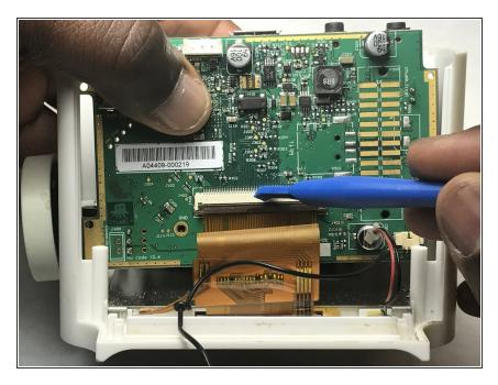
Remove the display ribbon cable from its socket with a plastic opening tool.
