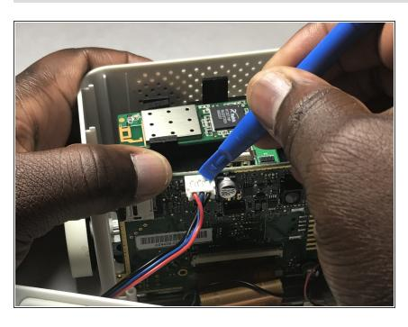
Disconnect the battery connector from the motherboard with a plastic opening tool.
