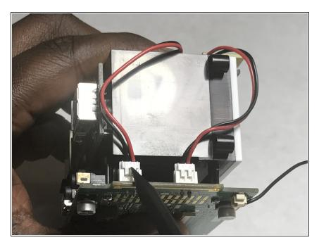
Remove the speaker connector using a plastic spudger.
