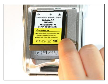
Pry up the battery from the bottom using a finger and remove the batter from the case.
