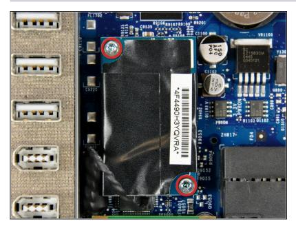
• Remove the two 5.5 mm T6 Torx screws securing the modem to the logic board.
