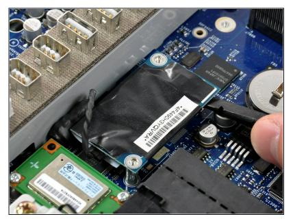
• Pry the modem straight up from its top edge to disconnect it from the logic board.
