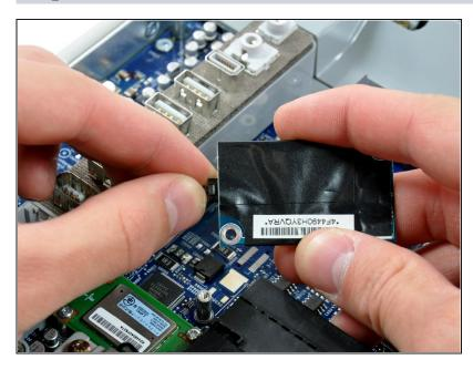
• Pull the modem cable connector straight away from the modem.
