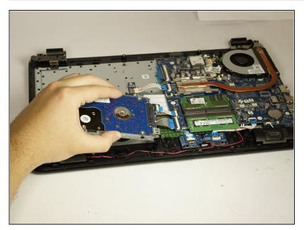
• Lift the hard drive out of its slot after screws are removed.
