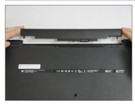
Pull the battery out of its slot.
