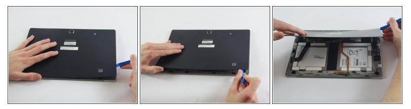
• Using the plastic spudger, open up the back of the device.
