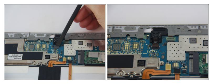
Using the black nylon spudger, flip the top half of the connecting port downward until you hear a click.
