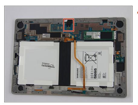
• Locate the camera and its corresponding connecting port.
