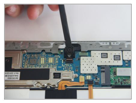
Proceed to lift up the camera out of its resting position.
