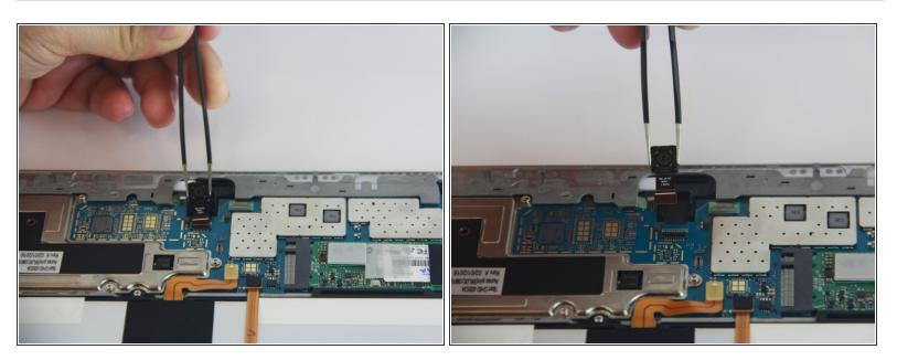
• Simply pull the camera parallel to the device out of its connecting port.
