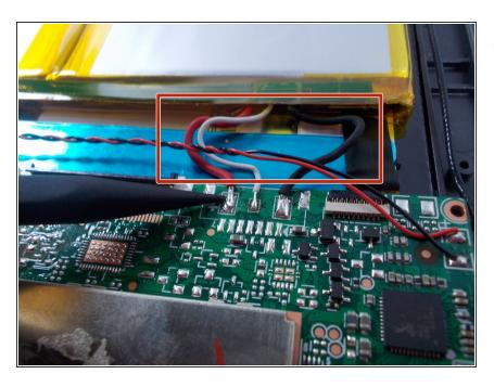
Splice the new battery with the red, white, and black wires connected to the motherboard.
