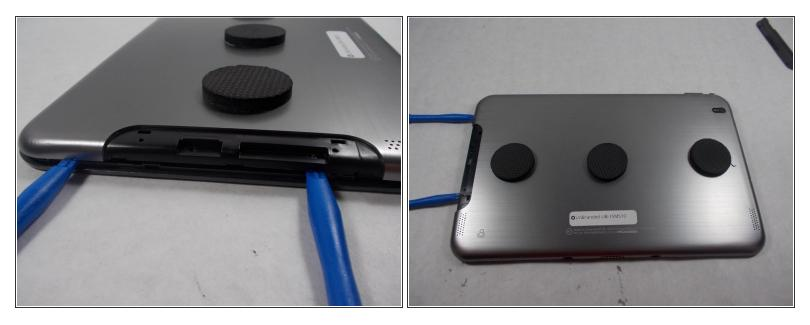
• Insert opening tools to partially pry open the cover.
