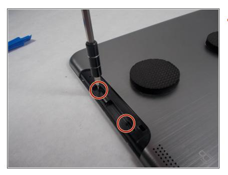
Remove the two 1.2 mm screws within the compartment using a Phillips #00 screwdriver.
