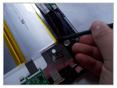
• Carefully remove the battery, making sure that all wires are disconnected.
