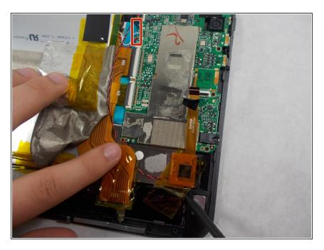
• Cut the wires connecting the battery to the device using a pair of wire cutters.
