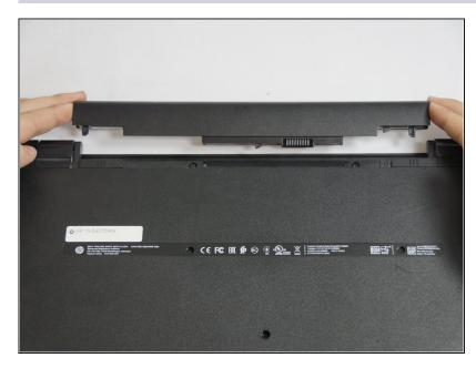
Pull the battery out of its slot.
