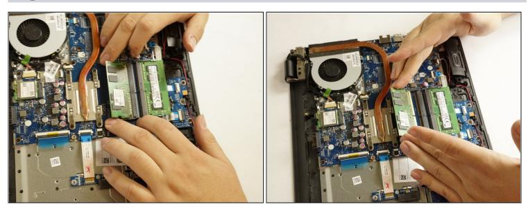
• Once the module is released, gently pull the module upwards.
