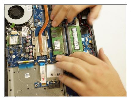
Push the two metal tabs on the side of the RAM module outwards, towards the battery and CMOS compartments (up and down).
