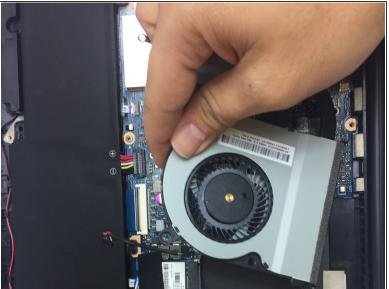
Once all screws and the connector are removed, you can safely pull the fan out of its place.
