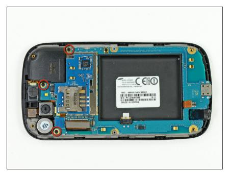
Remove the three Phillips screws securing the motherboard to the front display assembly.
