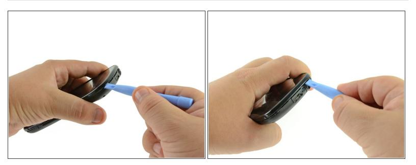
In the same manner as previously described, release the bottom clips located near the bottom of the Nexus S.
