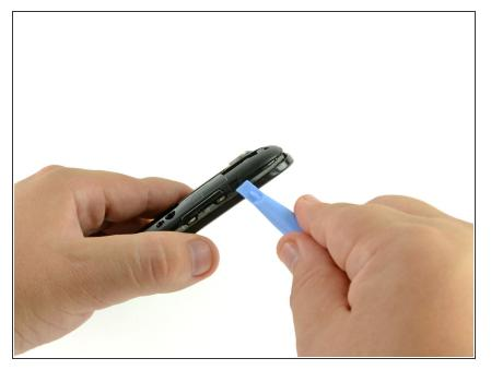
Insert and pry the plastic opening tool to release the final clip securing the rear inner frame to the inner assembly.
