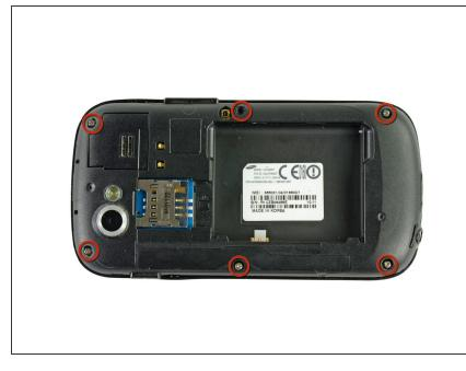
Remove the six Phillips screws securing the rear inner frame to the inner case.
