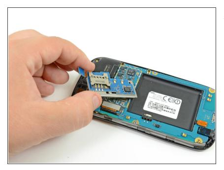
• Lift and remove the SIM Card board out of the Nexus S.
