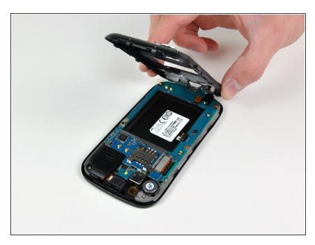
• Lift and remove the rear inner frame from the Nexus S.
