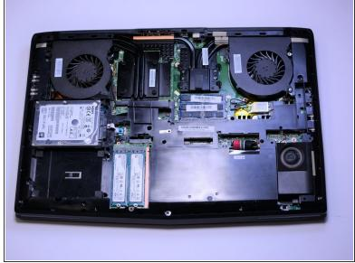
Lift the back cover using the tab to expose the hardware beneath.
