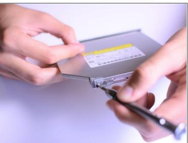
Remove the indicated 4mm Phillips #0 screw and metal hinge.
