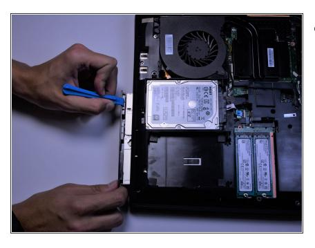
Using the plastic opening tool, pull out the CD drive.
