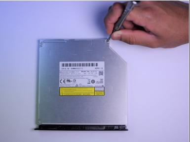
Remove the three (3) indicated 2mm Phillips #0 screws.
