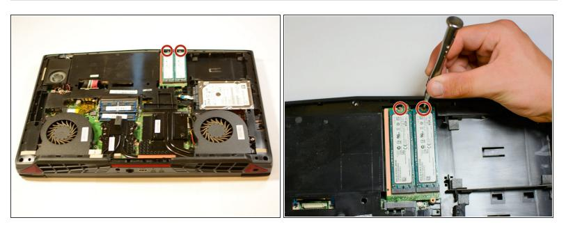
• Remove the two 6mm #0 Phillips head screws securing the two SSDs.
