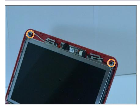
• Unscrew the two screws using a Phillips #00 screwdriver from the metal casing that retains the screen.
