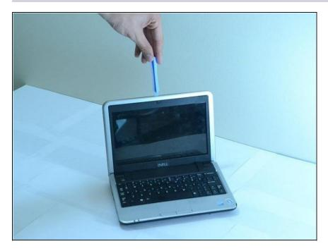
• Using a plastic opening tool, pry the front silver bezel away from the colored plastic shell.
