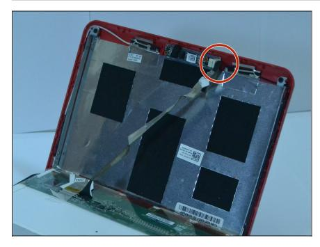
Gently lay the screen down, being careful not to damage the ribbon connector.
