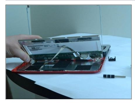
Disconnect the cord connecting the screen to the rest of the laptop. The cable will be attached to the screen using tape, so it can be safely removed. The actual cord connection is at the circuit board.
