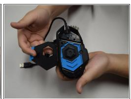
Remove the bottom panel of the device.
