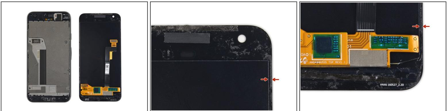
ⓘ In the following steps, you will separate the display panel by slicing through the adhesive bonding the display to the Pixel's chassis.
