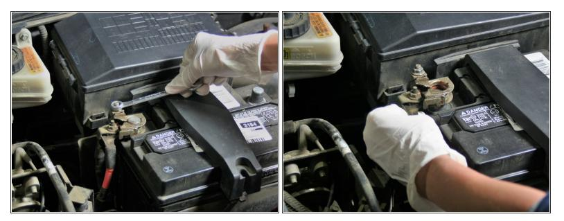
Remove the positive cable (usually red in color and labeled with + or "Positive")by turning the nut clockwise with the wrench.
