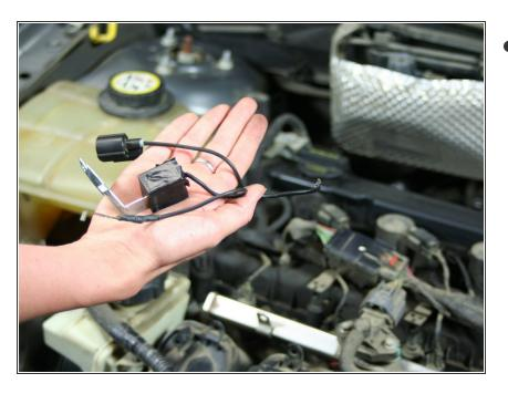
Obtain the new capacitor and reattach it by reversing the same steps you followed to disconnect the old capacitor.
