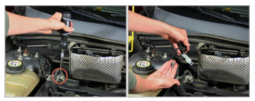
Unscrew the second anchor bolt that secures the metal mount.
