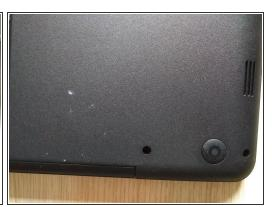
Remove the remaining screws on the bottom of the device.
