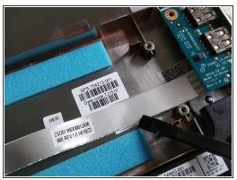
Use a spudger to loosen the cable from the bottom plate.
