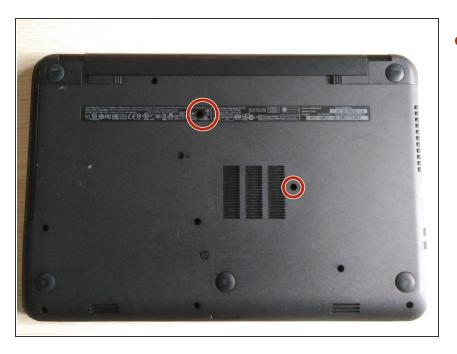
Remove the two indicated screws using a #1 Phillips driver.
