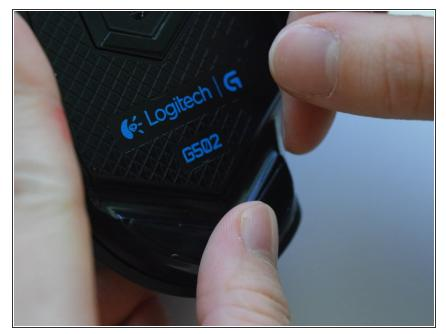
Apply even pressure across the mouse feet to ensure adherence.
