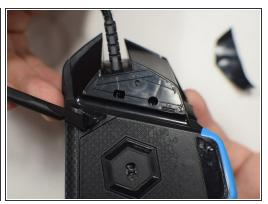
• Use your fingers or a nylon spudger to peel the old feet off all three corners where the screw holes are exposed.
