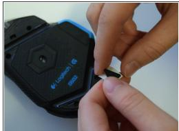
Peel the backing off the new mouse feet to reveal the adhesive.
