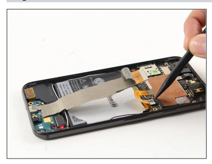
Use a spudger to disconnect the thin, black ribbon cable connecting the power and volume buttons to the motherboard.
