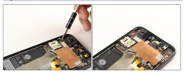
• Remove the two silver 2.5 mm T5 screws holding the motherboard in place.
