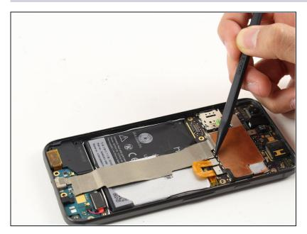
Using a spudger, disconnect the battery ribbon cable from the motherboard.
