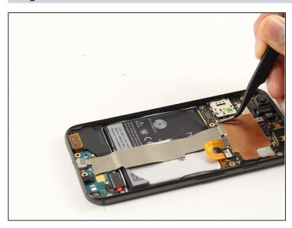
Use <u>tweezers</u> to lift up the adhesive strip at the top of the battery, and peel it back to expose the connector underneath.
