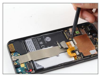
Use a spudger to disconnect the charging port ribbon cable from the motherboard.
