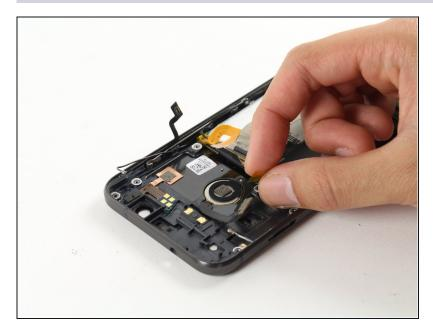
Pull the fingerprint scanner out of its housing.
