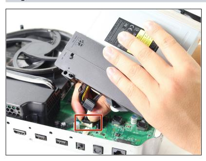
Pull the disc drive slightly off the motherboard and disconnect the plastic connectors from the motherboard.
