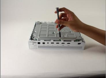
• Use a T10 Torx screwdriver to remove the six green 50 mm long screws from the metal case labeled F1 through F6.
