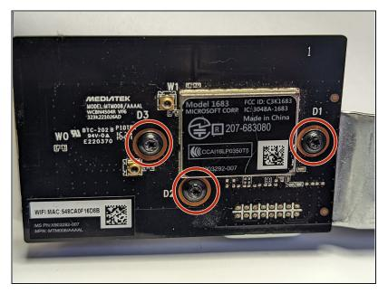
Remove the three black 8 mm T-9 Torx screws labeled "D1," "D2," and "D3" to remove the Mediatek board.
