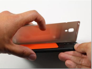
Run the plastic opening tool along the seam on the side of the phone to remove the rear casing.
