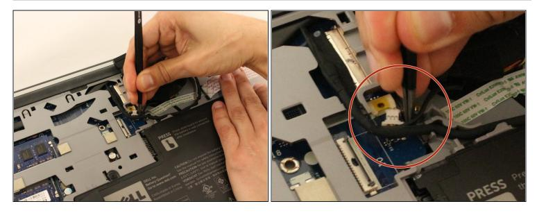
• Use <u>tweezers</u> to remove the small cable attached to the fan.
