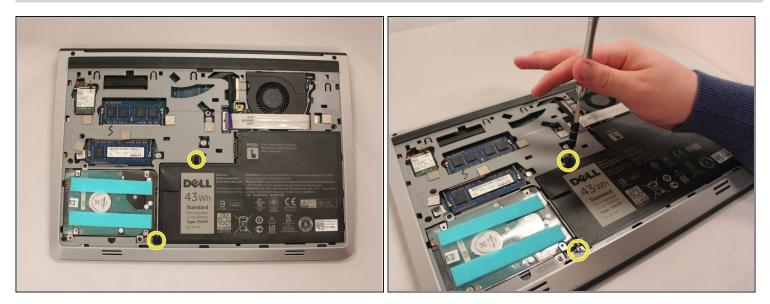
• Remove the two 5.70mm Phillips #0 screws that secure the battery in place on its left side .
