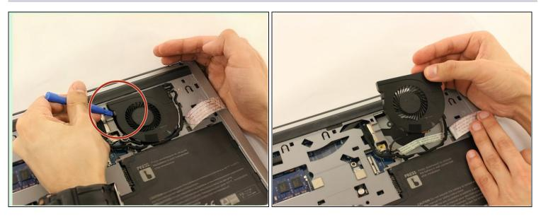
• Using the opening tool, pry the fan out.
