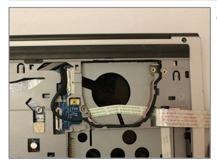
(i) Now that the fan is removed, be sure to clean the area under the fan to prevent overheating.
