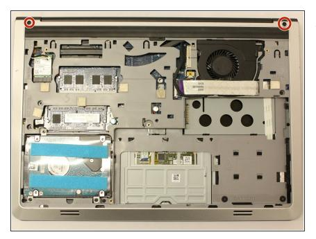
Locate the two black (8.70mm) screws at the laptop's hinges and unscrew.
