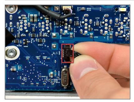
• Disconnect the ambient light sensor by pulling its connector up off the socket on the logic board.
