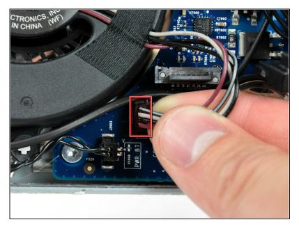
• Disconnect the CPU fan by pulling its connector up off the logic board.
