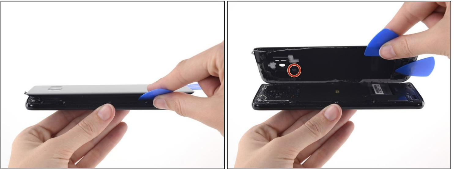
**i** The fingerprint sensor cable connects the phone to the rear glass near the main camera. The cable is very short and should disconnect as the rear glass is removed.
