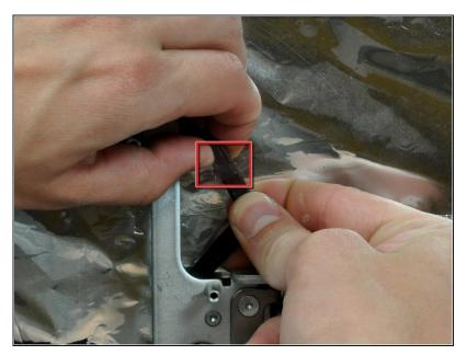
Disconnect the AC-in connector by simultaneously squeezing the lock mechanism and pulling the connector away from its socket.
