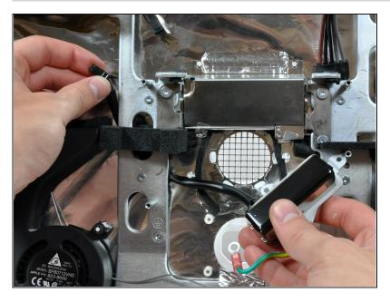
De-route the AC-in cable from beneath the chassis.
