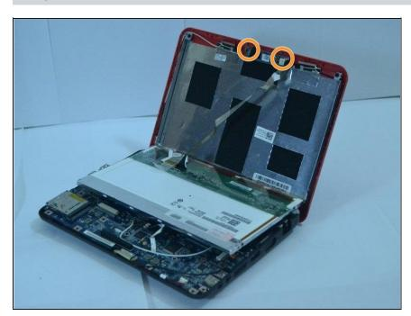
Replace and tighten the two screws so that the module is held in place.
