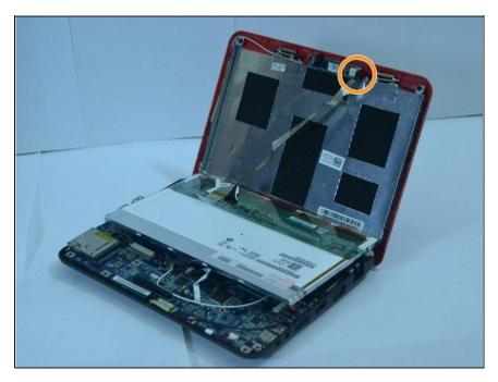
Carefully connect the ribbon cable running along the back of the screen to the appropriate docking station in the webcam module.
