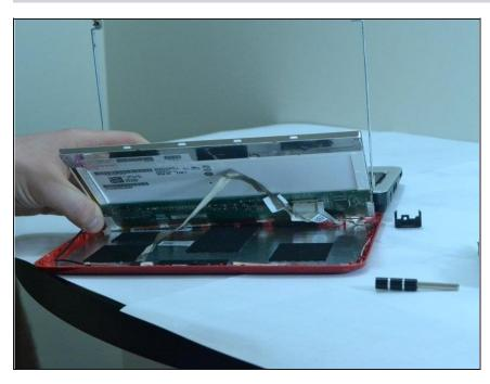
Disconnect the cord connecting the screen to the rest of the laptop. The cable will be affixed to the screen using tape, so it can be safely removed. The actual cord connection is at the circuit board.
