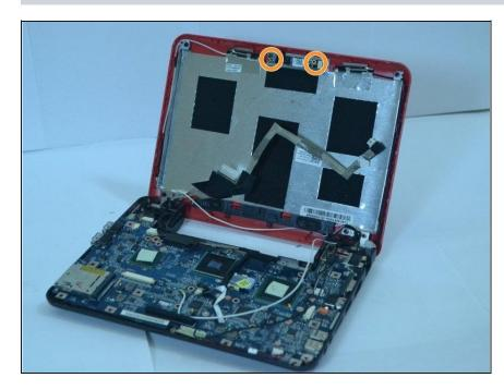
Remove the two small screws above the screen at the center of the lid.
