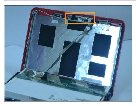
Insert the replacement webcam module so the two screws match up with the two holes in the module.
