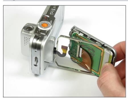
• Pull the screen away from the camera the same way that you removed the screen backing.
