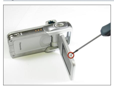
Remove the screw(2.6mm
