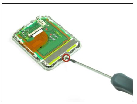
• Use the screwdriver to remove the screw(2.46mm Philips) indicated.
