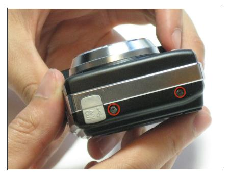
Remove the two 3.0mm screws on the right side of the camera.
