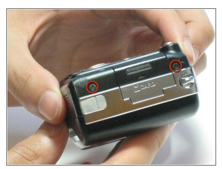
Remove the two 3.0mm screws on the left side of the camera near the memory card compartment.
