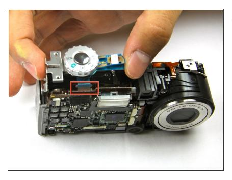
Remove the top button piece. You will need to detach a small blue ribbon cable before the button can be fully removed.
