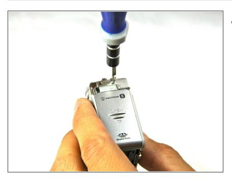
Remove the 3.0mm Phillips #000 screw above the battery door on the side of the camera.
