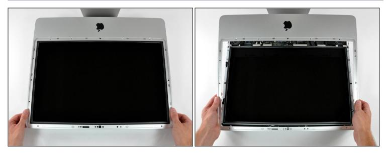
$\triangle$  The front bezel is still attached to the iMac by the microphone cable.
