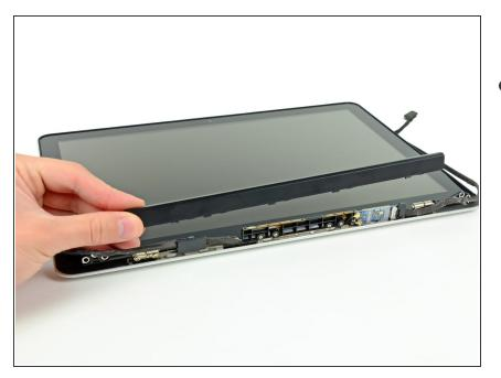
Remove the clutch cover from the display.
