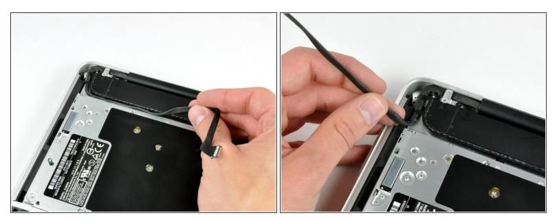
• De-route the camera data cable from the channel in the optical drive.
