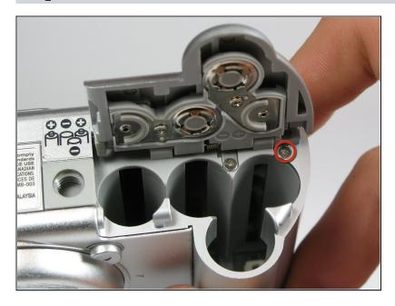
• Remove the rightmost 4.2mm screw underneath the battery cover, not the center screw.
