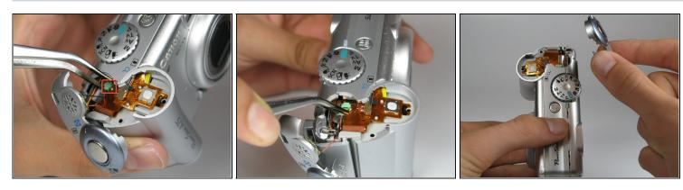
• Using a pair of tweezers, grab the plug that connects the speaker to the camera and gently pull it out.
