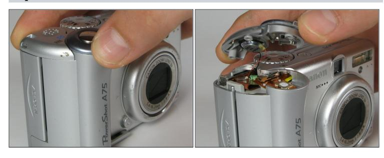
• Lift the shutter button and speaker part from the top of the camera.
