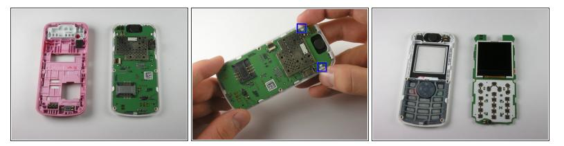
• Put the red casing aside and remove the motherboard from the front casing of the phone by carefully dislodging it from its two clips near the top of the phone.
