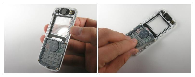
• As you can see, the rubber keypad is attached to the front casing. Gently remove it from the case by pinching any part of it and lifting. Don't worry, it isn't attached too firmly and is easily removable.
