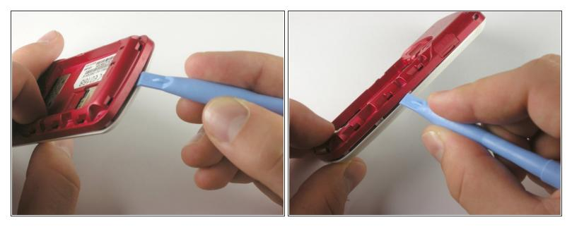
• Using the plastic opening tool, pry open the body of the phone, starting at the bottom of the phone (this tends to be the easiest place to start).
