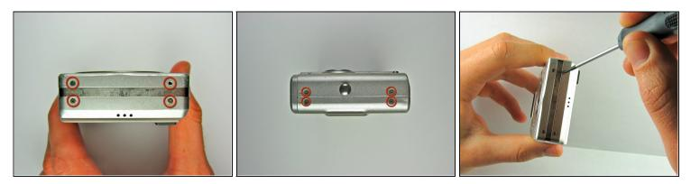
Remove eight 1.8 mm screws from the left and right sides of the camera using a Phillips #00 screwdriver
