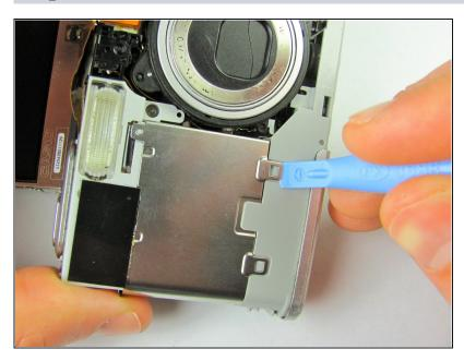
• Using the iFixit plastic opening tool, pry the battery case clamps on the front of the camera so that the bottom will come loose.
