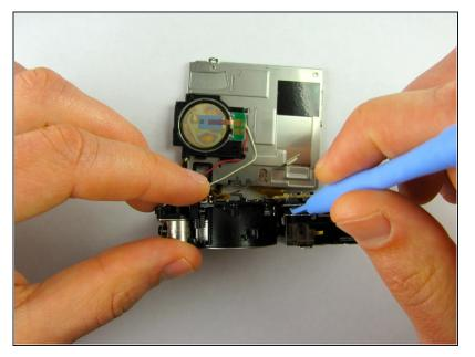
Detach the inner orange ribbon cable that connects the motherboard to the lens by inserting the iFixit plastic opening tool under the tab and lifting up.
