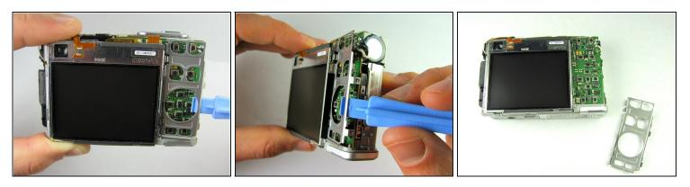
• Remove the metal grating located to the right of the LCD screen by inserting the plastic opening tool under the grating and pulling up.
