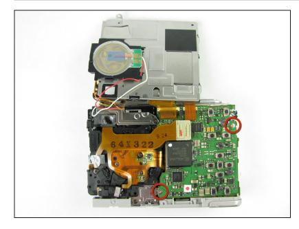
Remove the two 1.7 mm screws from the motherboard using a Phillips #00 screwdriver.
