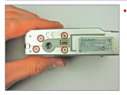
• Remove the four 3.7 mm screws from the bottom of the camera using a Phillips #00 screwdriver.
