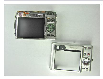
• Separate the back case from the body of the camera.
