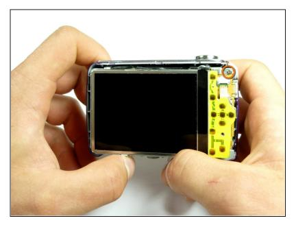
• In the top right hand corner of the inside of the camera, there is a Philips #00 4 mm screw that needs to be removed.
