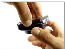
Once all the screws are out, remove the back panel.
