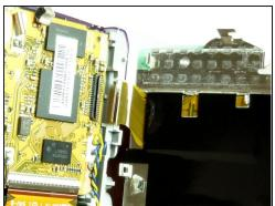
• To remove the screen completely, push down on the rectangular tab indicated in the picture.
