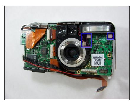
Disconnect the two wired plugs below the flash.
