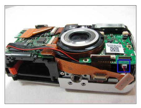
Disconnect the wired plug at the bottom of the right motherboard.
