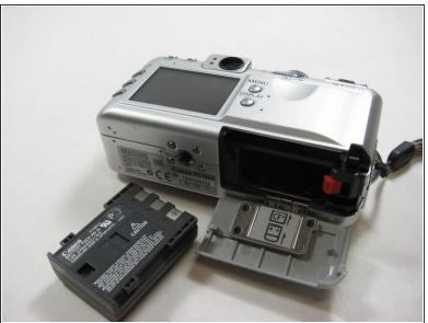
Holding the edges, slide out the battery.
