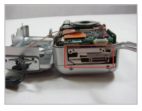
Use a pair of tweezers and remove the metal piece inside the camera.
