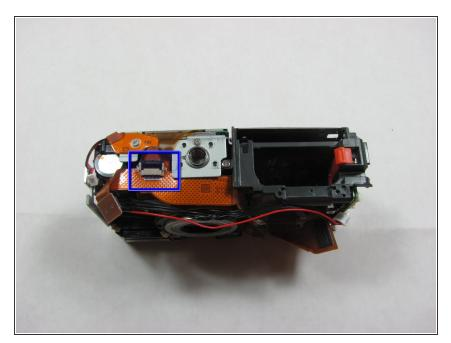
Disconnect the film from the bottom of the camera under the LCD Screen.
