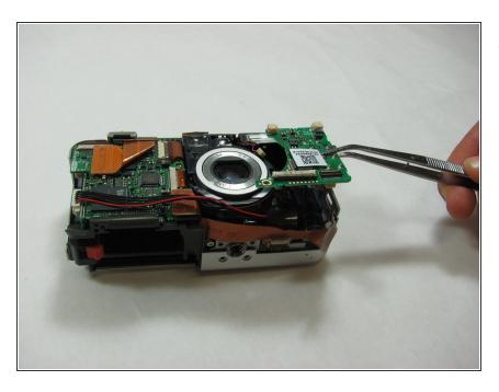
Use a pair of tweezers to pull the right motherboard away from the main body of the camera.
