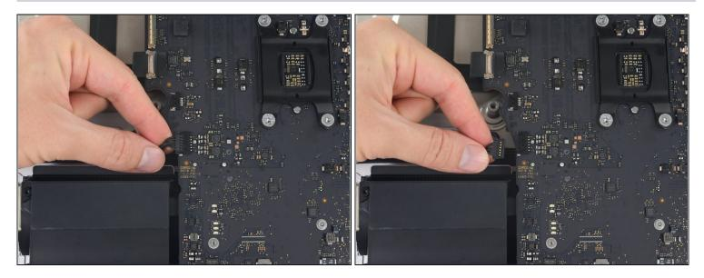
• Gently pull the left speaker cable straight out of its socket on the logic board.
