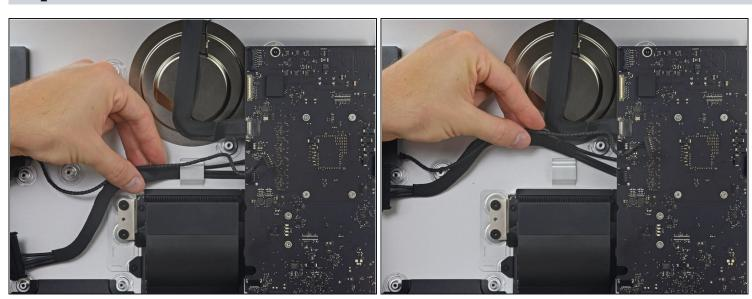
• Similarly to the previous step, de-route the SATA and power cables by pulling the braid straight up out of the retaining clip.
