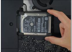
• Lift the hard drive from the edge nearest the logic board and pull it slightly out of its recess.
