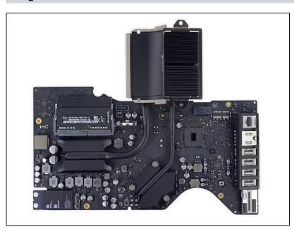
Handling the board by the edges, flip the logic board over to access the two RAM modules.
