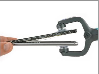
Use an iSclack or a suction handle to separate the display unit from the rear case.
