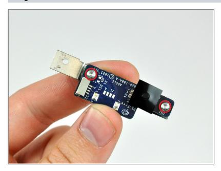
Transfer the two T6 Torx screws and the IR bracket to your new IR board.
