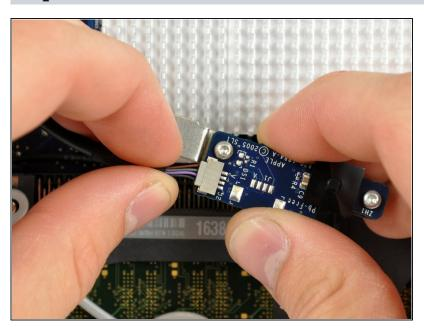
Pull the IR Board cable connector straight away from its socket on the IR board.
