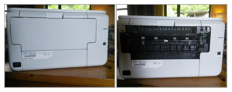
Stick your printer on a table and get to the back of it. Then remove the white flap from its hinges.
